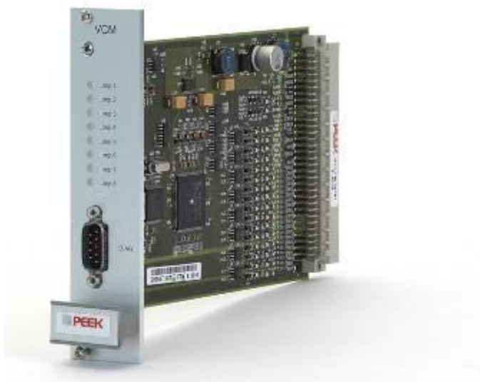
Figure 33 Layout VECOM Control Module (VCM)
